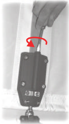
Turn adjuster clockwise on the Sailman batten box to tension batten
